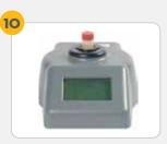
The fdMplus tests for metallic ferrous wear metals in lubricants and greases. Test in seconds, in the bottle, to give immediate pre-warning of
